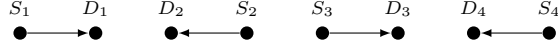
Fig. 14. Configuration of unicast sessions, used to achieve \lceil L/2 \rceil symbols×hops per time slot under P/P.
