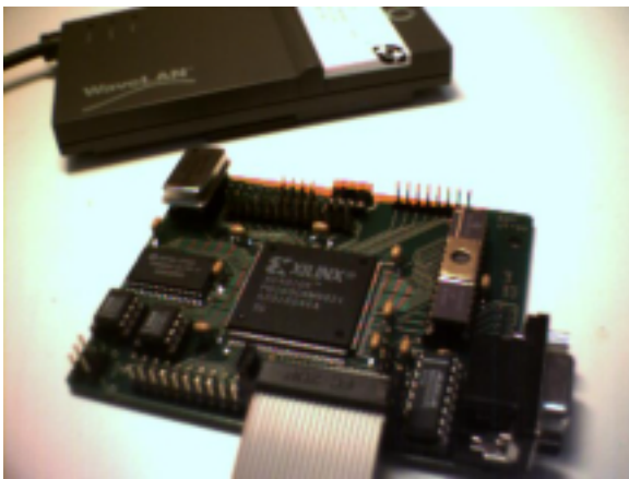
Figure 8: Network interface implementation.
