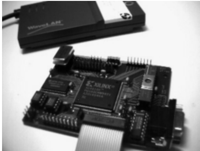
Figure 6: Network interface implementation.
