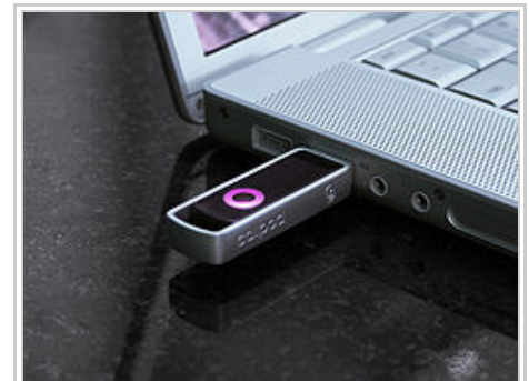
A Bluetooth USB dongle with a 100 m range. The MacBook Pro, shown, also has a built in Bluetooth adaptor.
