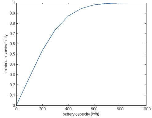
Fig. 6. The minimum of the survivability level as a function of the back-up capacity for the winter scenarios.
