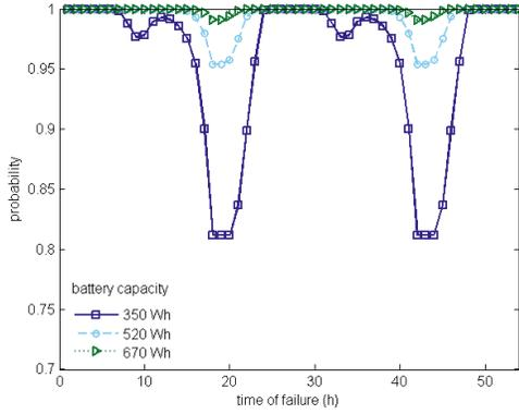
Fig. 5. The probability of surviving a grid failure as a function of the time that the failure occurs for the winter production and demand profiles.
