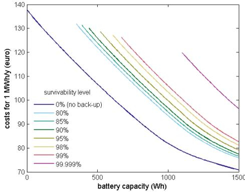
Fig. 11. Costs for 1 MWh/y electricity as function of the installed battery capacity for different survivability levels.
