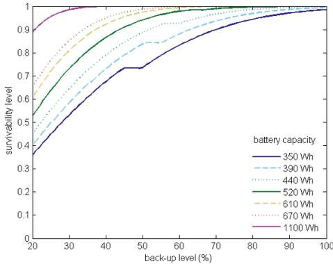
Fig. 9. Achievable survivability level for different battery sizes as a function of the backup level in summer.
