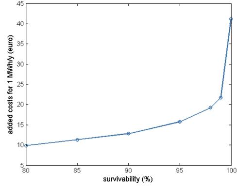
Fig. 12. The additional costs to obtain a given survivability level compared to the situation with no back-up capacity for a 1100 Wh battery.
