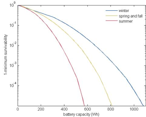
Fig. 7. (1 - the minimum of the survivability level) as a function of the back-up capacity for the three season scenarios.
