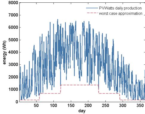
Fig. 2. Energy produced per day according to the PVWatts profile, and an indication of the worst case level.
