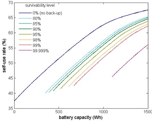
Fig. 10. Self use rate as function of the installed battery capacity for different survivability levels.
