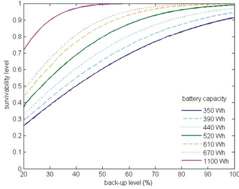
Fig. 8. Achievable survivability level for different battery sizes as a function of the backup level in spring-fall.
