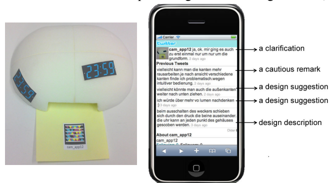
Figure 3: Foam model of an alarm clock with 2D barcode and its Tweet log showing different activities.
